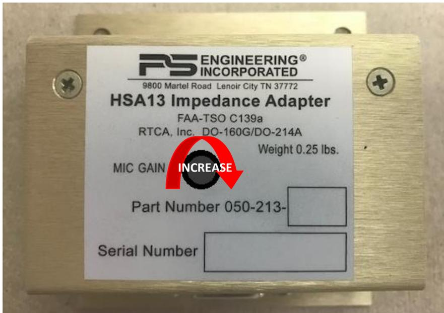
**Figure 2-1 Microphone Gain Adjustment**
