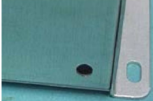
Figure 2-10 Radio Output Level Adjustment
