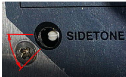
Figure 2-9 Sidetone adjustment range
