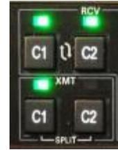
When you want to transmit on COM 2, just push the C2 XMT button, and both indicators will switch over.
