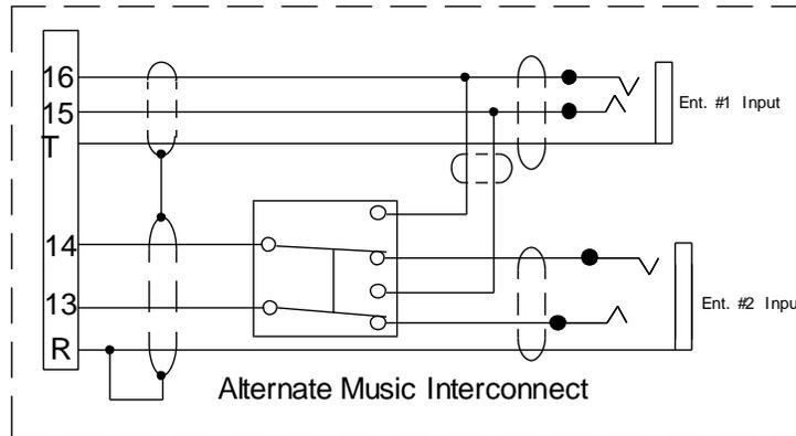
**NOTE:** Use the low level output of any additional entertainment device to connect to the audio panel. Maximum signal level is **2 VAC** p-p. **DO NOT** use a speaker-level output, this will cause internal damage in the audio panel.
