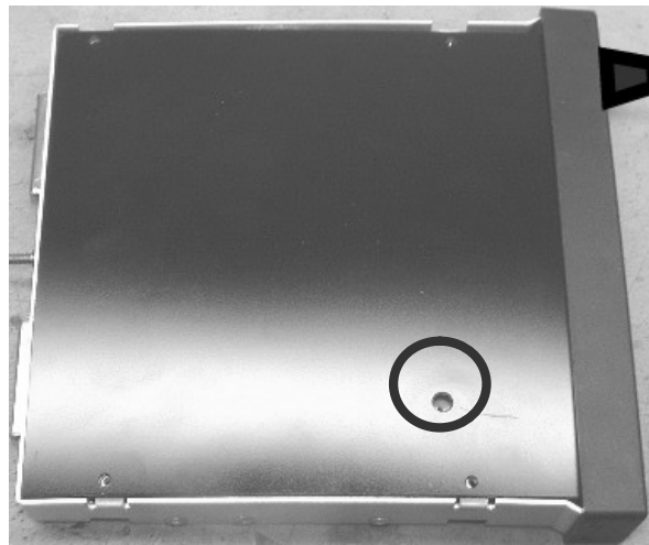
Figure 2-3 – Unswitched 3 Audio Level (bottom cover removed)
