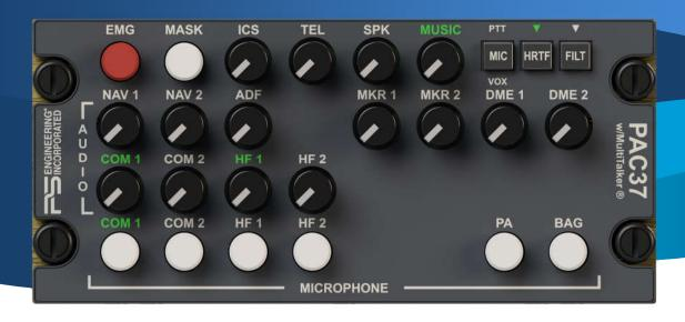
PS Engineering's Configuration Tool and fully customizable label nomenclature ensures the PAC37 will replicate the functionality of the existing audio system.
